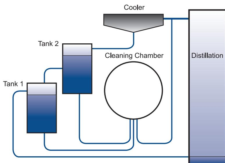
1. Pre-washing – flooding of the cleaning chamber with solvent from tank 1.
